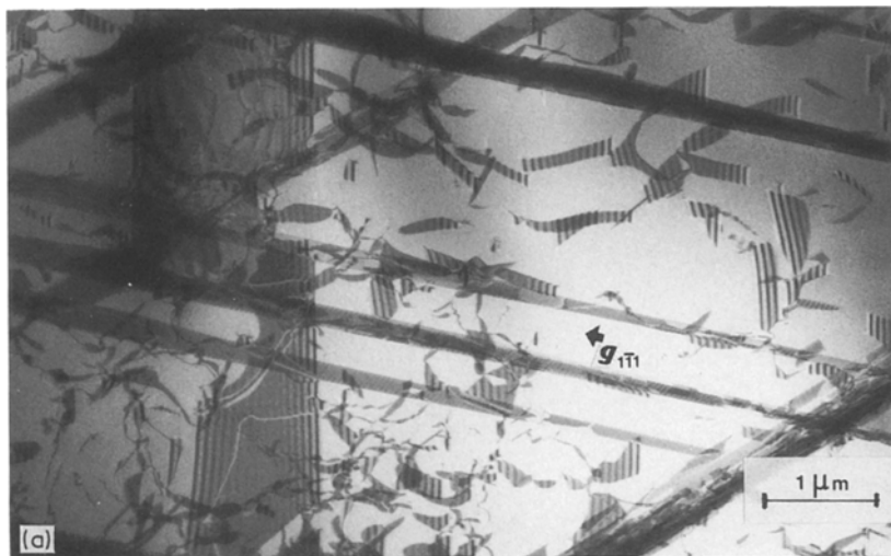
Figure 2 Transmission electron micrographs showing the effects of nickel additions on the structures of dissociated dislocations, stacking faults and twins in the as-cast Co-Cr-Mo alloy. (a) The base alloy, (b) the alloy with 4 wt % nickel, and (c) the alloy with 9 wt % nickel.
